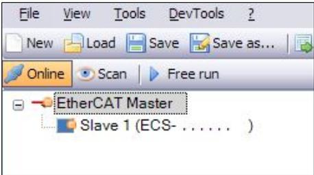
Figure 4: Scan result showing “Slave 1 (ECS-PMC/FPGA)”, (picture detail)
